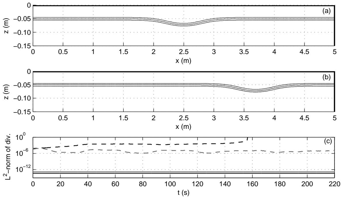
Figure 4: The position of the thin pycnocline is indicated by three contour lines of non-dimensional density  $\rho$  for the DJL ISW test case at times (a)  $t = 0$  s and (b)  $t = 540$  s using the  $N = 8$  WLP method. Panel (c) shows the  $L^2$ -norm of divergence vs. time for the methods:  $N = 4$  WLP (black, solid),  $N = 4$  NLP (black, dashed),  $N = 8$  WLP (grey, solid), and  $N = 8$  NLP (grey, dashed).
